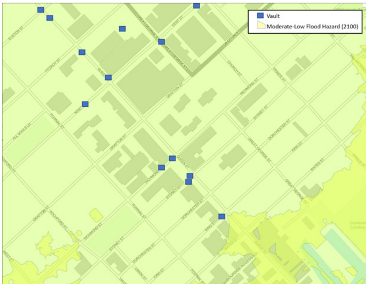
Figure 12: Year 2100 Flood Hazard Map with Maritime Electric Downtown Charlottetown Vaults
