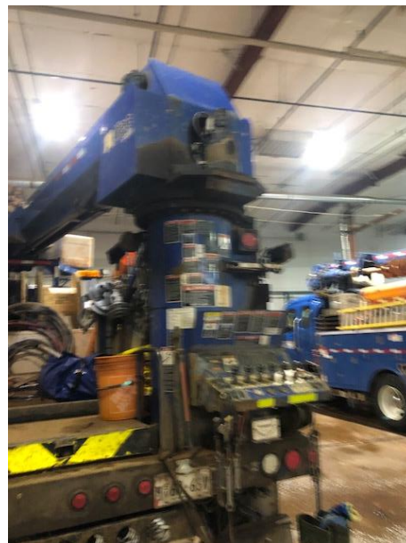
Truck 14-12-64 Turret for digger/derrick and control station
