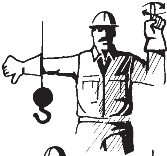
LOWER THE BOOM AND LOWER THE LOAD - Arm extended, fingers closed, thumb pointed downward, other arm vertical, forefinger pointed upward and rotate hand in horizontal circles.
