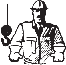
RETRACT BOOM - (telescoping boom) Both fists in front of body with thumbs pointed toward each other.
