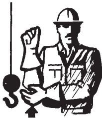
USE WHIPLINE - (auxiliary hoist) Tap elbow with one hand, then use regular signals.
