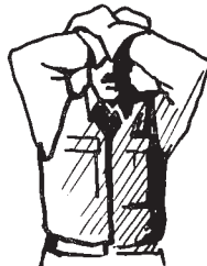
HOIST SLOWLY TO CLEAR FOULED LINE - Hands crossed in front, above shoulders, fingers relaxed.
