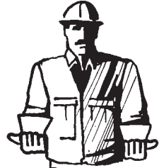
EXTEND BOOM - (telescoping boom) Both fists in front of body with thumbs pointed upward.
