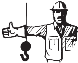
RAISE BOOM - Arm extended, fingers closed, thumb pointed upwards.
